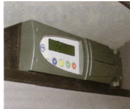
A Euroscan X1 Generation Recorder that was modified to meet the special communication needs at MCS.
